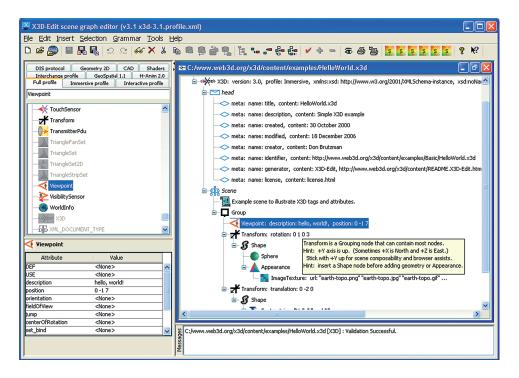
Figure 1.7. X3d-Edit is an XML-based Java application for creating and launching X3d scenes.
