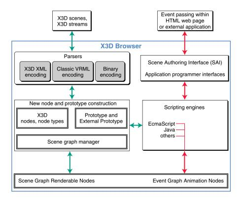
Figure 1.1. Example software architecture for an X3D browser.
