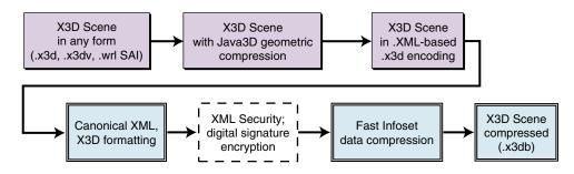
Figure 1.6. Processing chain to start with any X3D content, apply geometric compression (if desired), add XML security features (if desired), and produce .x3db compressed binary encoding.
